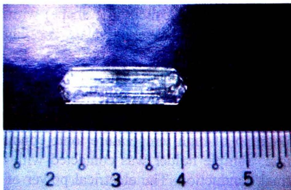
Figure.1 Photograph showing the as-grown crystal of  $\text{ZnSO}_4 \cdot 7\text{H}_2\text{O}$
